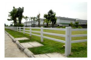
**4.3 Jambo fences** has a sheet size, width 125 cm. X length 290 cm. X thickness 6 cm., Consisting of 2 fence panels (including lintel), 3 meters from pole to pole, suitable for fencing housing projects Government offices, residential houses, industrial factories
